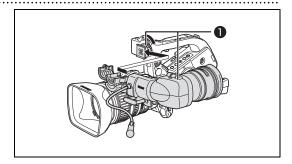
2. Connect the viewfinder cable to the EVF1 socket on the camcorder.
